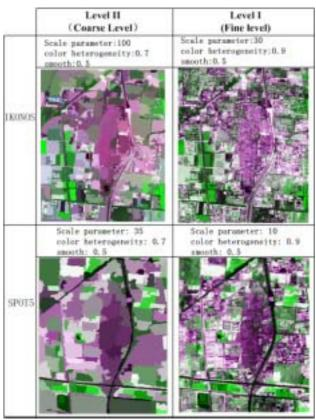
Figure 2. Multiresolution segmentation results of IKONOS and SPOT5 data
