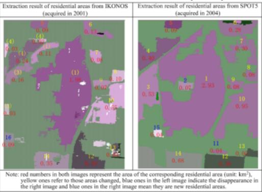
Figure 5. Change detection of residential areas based on the classification results of the two data
